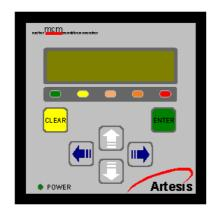
Artesis' revolutionary Motor Condition Monitor (MCM) uses the techniques of experimental modelling to assess and monitor the condition of electrical motors. Using only current and voltage signals, MCM can predict electrical and mechanical failures in both the monitored electric motors and any systems that may be connected to the motor. Detectable conditions include faulty bearings, misalignment errors, load imbalance and both rotor and stator faults.
